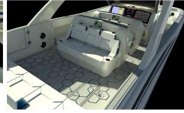
With a beam of 13', the 499 Sport is poised to become the industry's hottest luxury center console. It will feature up to three rows of seats, a full-length sun pad in front of the console, full forward seating, and full stateroom with full stand-up head and galley area inside the console. This boat will hold over 900 gallons of fuel.
